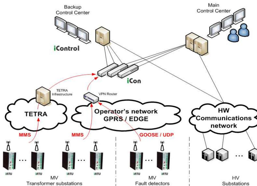
Figure 6. Use of data concentrators for MV information.
