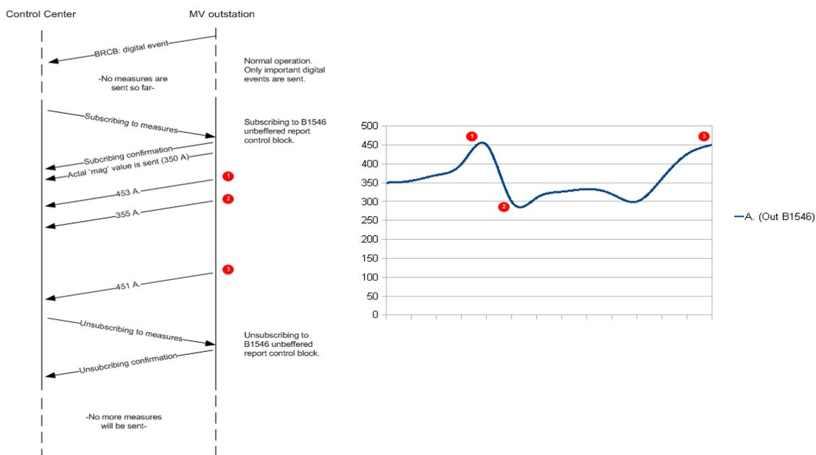
Figure 2. Measures on demand using IEC-61850
