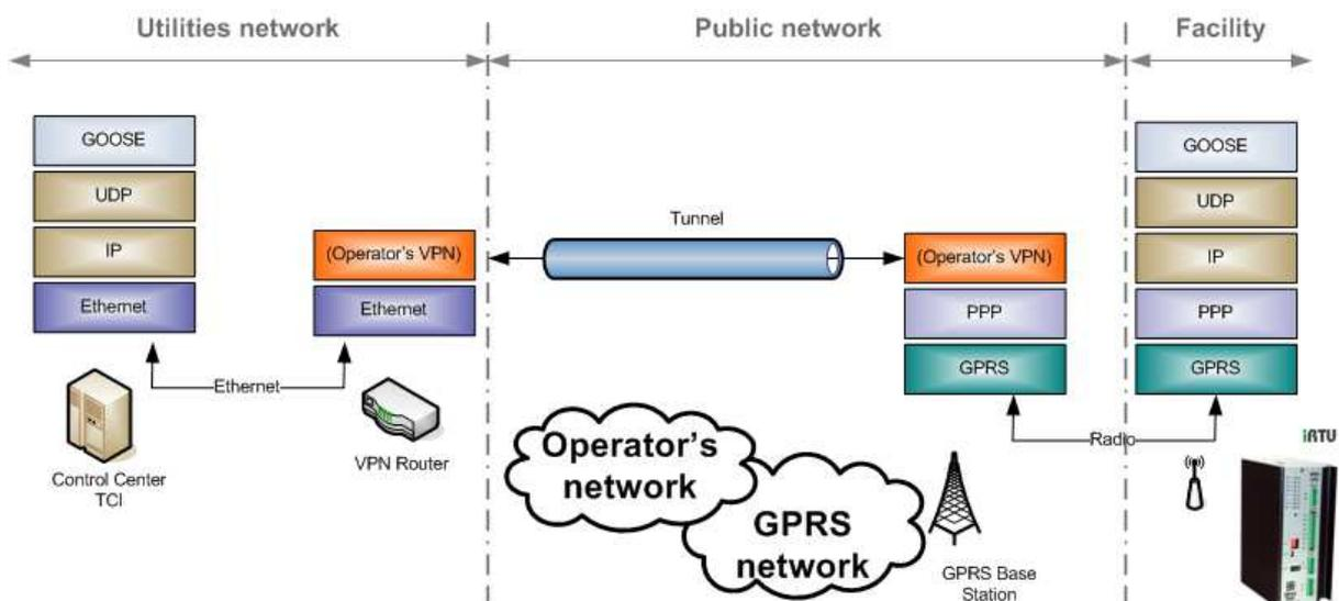
Figure 5. Protocol stacks used for GOOSE on MV.
