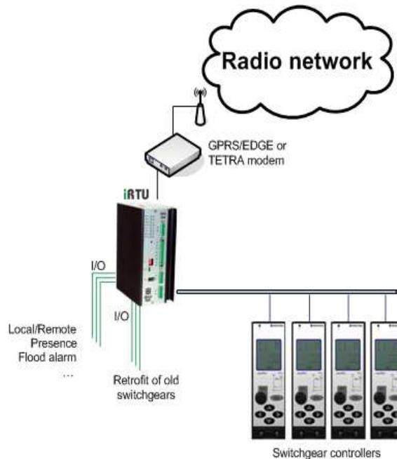
Figure 3. Use of an iRTU to integrate all information collected in a transformer substation.
