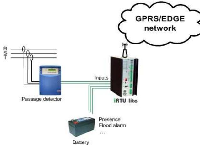
Figure 4. Power grid fault detection using iRTU.
